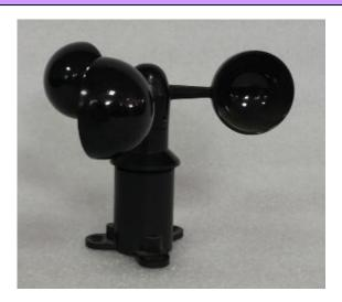
Wind Speed Sensor is designed with rugged components stand up to hurricane - force winds, yet are sensitive to a light breeze. Includes sealed bearings for long life. The range and accuracy specifications have been verified in wind - tunnel tests. In areas where icing of the anemometer is a problem, drip rings deflect water from the joint between moving parts.
